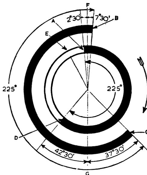
Valve timing diagram—Engine type Six-346
