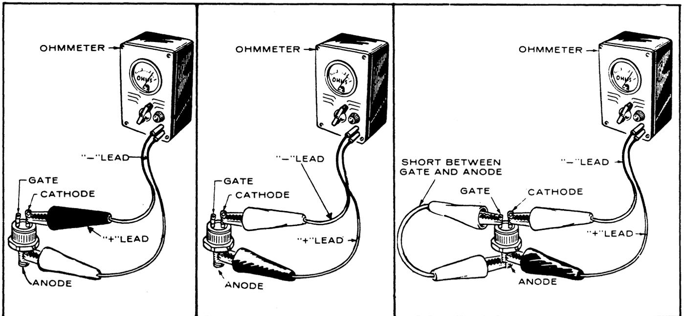
FIGURE 9. TESTING SCR's
