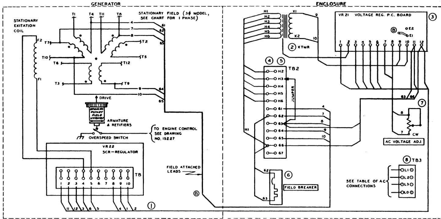
30 & 45KW: VOLTAGE REGULATOR & POWER CONNECTIONS
