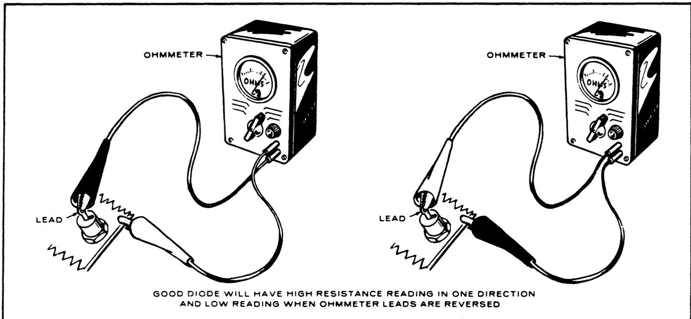
FIGURE 8. TESTING DIODES
