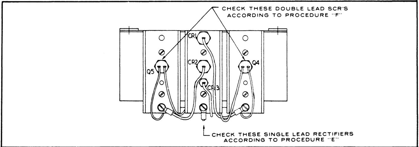
FIGURE 3. TOP VIEW OF EXCITER-REGULATOR CHASSIS ASSEMBLY
