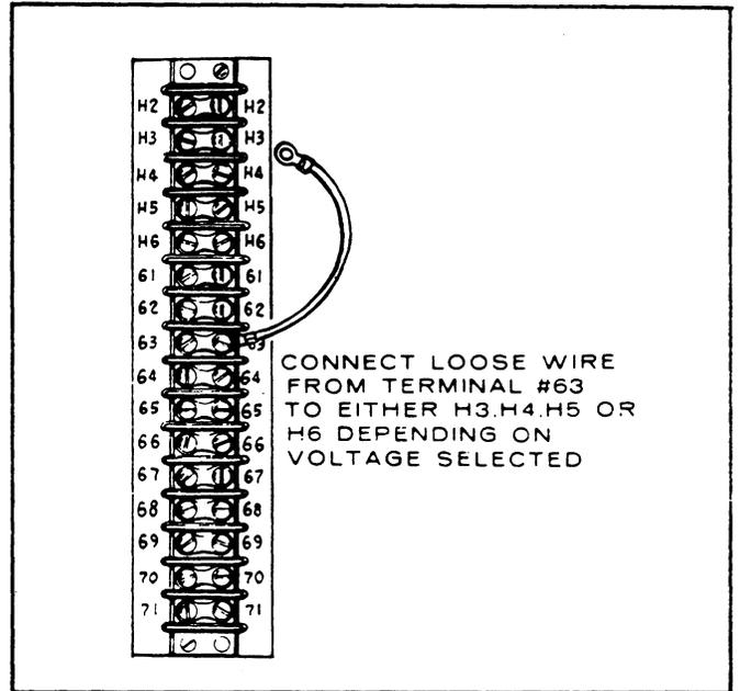
FIGURE 23. CONNECTING LEAD FROM TERMINAL 63
